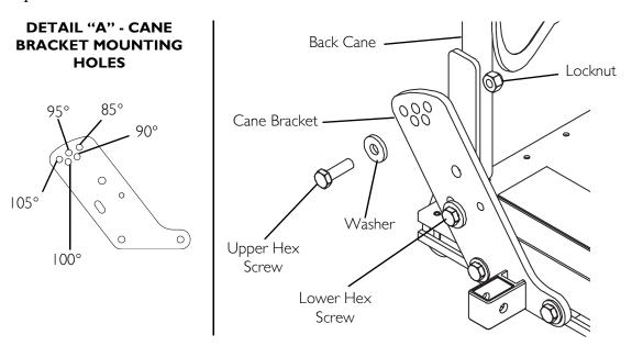
FIGURE 8.1 Adjusting the Back Angle
